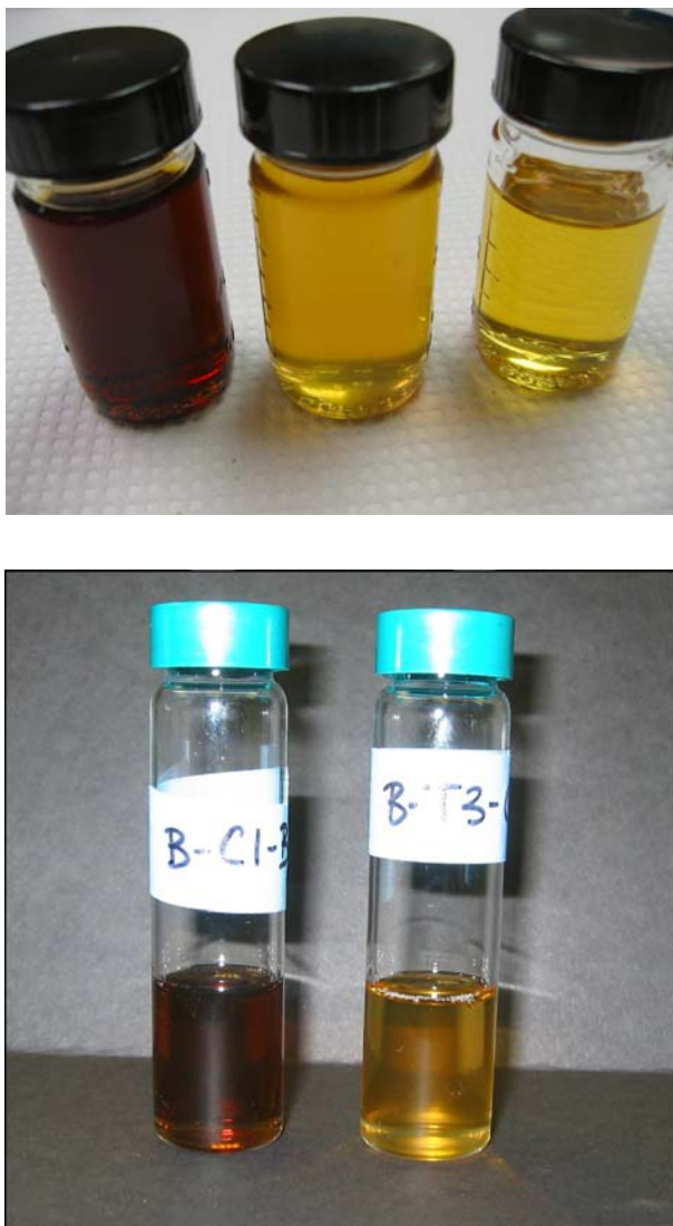
FIGURE 4.10 Effect of treatment of syrup with decolorizing resin (Top: from left to right, control syrup, decolorized, further decolorized) and hydrogen peroxide (Bottom: control syrup, treated syrup).
